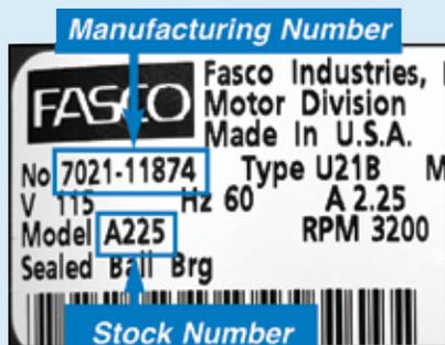
Just a reminder...when you or your customer is trying to find the right replacement for a Fasco OEM product, the Fasco part/manufacturing number on the nameplate is the key. Our OEM motors and blowers are numbered with an 8-digit (occasionally 9) manufacturing number, such as 7126-1672. The first two digits are always 70 or 71, depending on what type of product Fasco provided:
